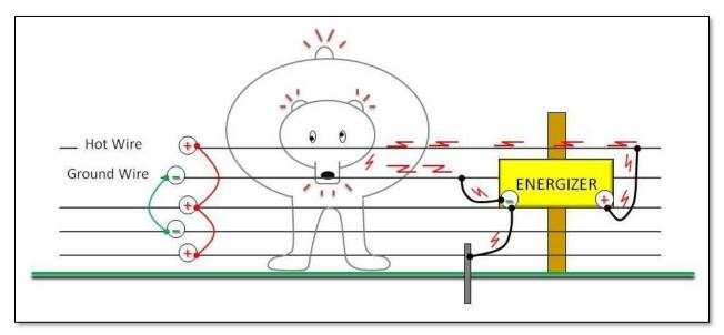
Figure 3. A ground-return electrified fence design. All hot wires are connected to each other in series and to the positive terminal on the energizer. All ground wires are connected to each other and to the negative terminal on the energizer. The negative terminal of the energizer is also connected to a grounding rod.
