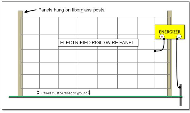
Figure 6. Electrified rigid wire panel. The panel is raised off the ground and insulated by hanging it from fiberglass posts. The wire panel is electrified by connecting it directly to the positive terminal on the energizer. The ground rod is connected to the negative terminal of the energizer.
