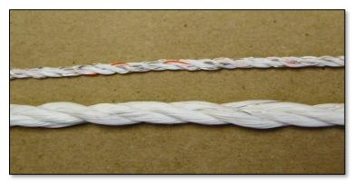
Figure 4. Two different styles of 9-stranded Polywire
